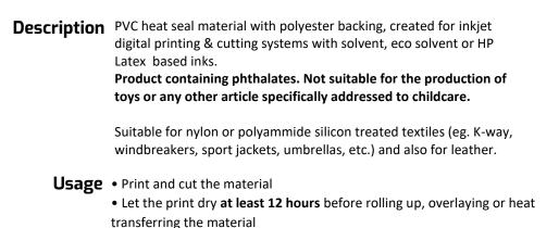
When printing on HP Latex plotter, set the drying temperature at 90°C
