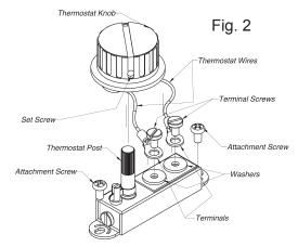
4. Plug machine in and turn the power switch "on" If heat light comes on, and the machine starts heating, replace thermostat.
