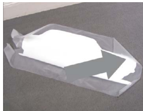
Peel back Release Liner from graphic. Pull in one direction holding down graphic
