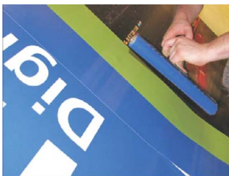
Always apply from center out using firm pressure on the roller.
