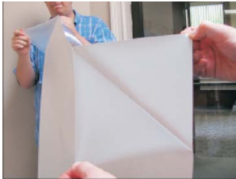
Peel back a few inches of release liner to create a hinge.
